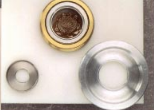
Fig. 10. After bombardment. Disassembly of the chamber components reveals that the helium pressure has forced the macrocarrier from its holder (now empty, bottom left) onto the stopping screen. Note the imprint of the screen on the macrocarrier.
