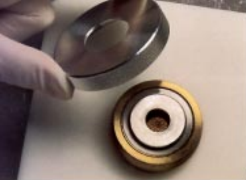
Fig. 9. Microcarrier launch assembly. Once the microcarrier slurry is completely dry, the holder is inverted (such that the microcarriers face the target cells) and placed into the microcarrier launch assembly. Note the stopping screen near the bottom of the assembly.
