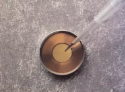
Fig. 8. Loading DNA samples. The DNA-coated microcarriers are pipetted onto the macrocarrier seated in the macrocarrier holder.
