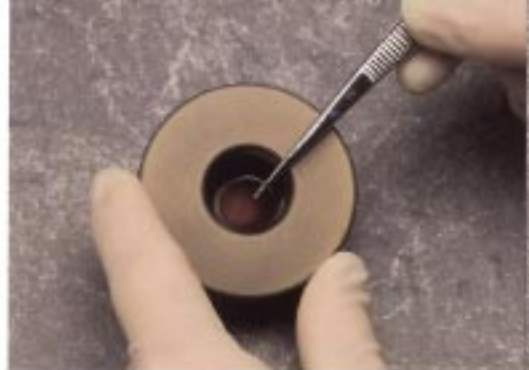
Fig. 7. Inserting rupture disk. An appropriate rupture disk is chosen and placed into the rupture disk retaining cap. Next, the cap is tightened onto the end of the gas acceleration tube.
