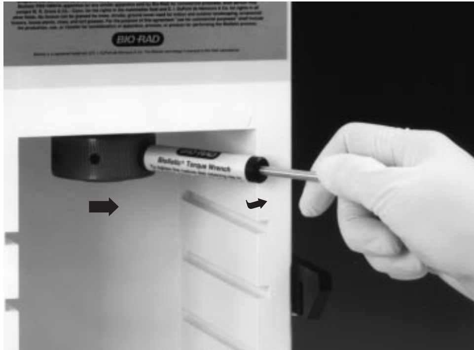
Fig. 4.8. Proper torque applied to retaining cap with torque wrench.
